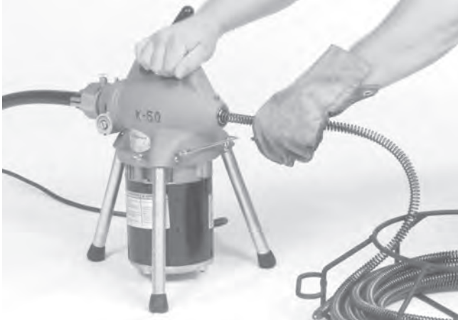
Figure 3 – Inserting Cable Into Front Of Machine
