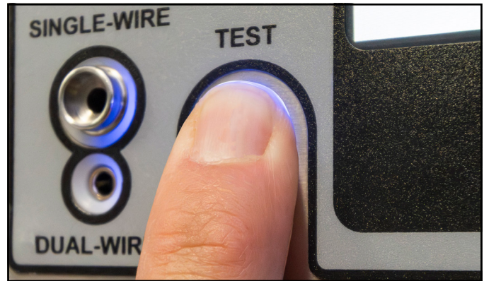
Figure 25. Bridging the test switch's contacts
