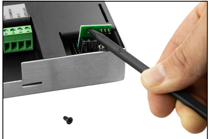
Figure 30. Lifting the used dual-wire wrist strap jack from the SmartLog
