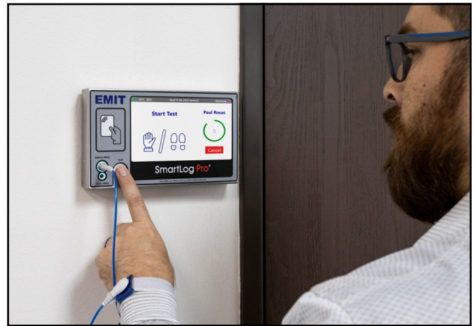
Figure 26. Performing a single-wire wrist strap test
