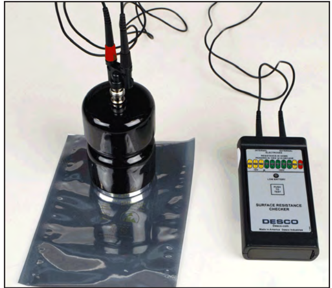
Figure 4. Using the Concentric Ring Probe with the Desco Surface Resistance Checker
