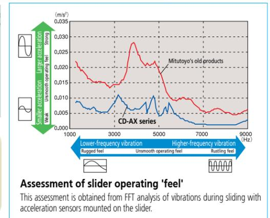
The slider provides **smooth, stable and comfortable operation**.
