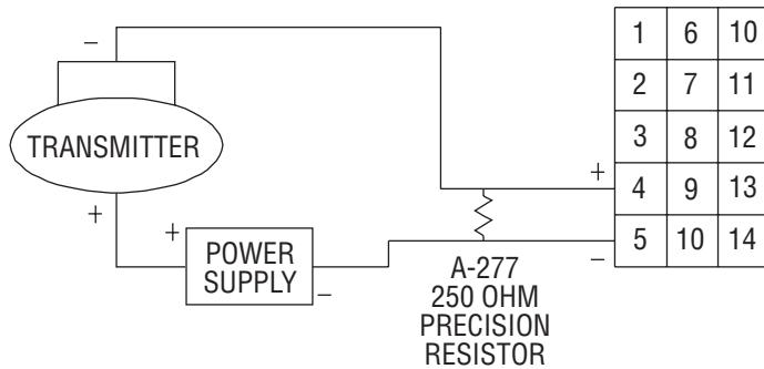
Note: 16B terminal layout used in above example. Use appropriate terminal layout for selected controller.
