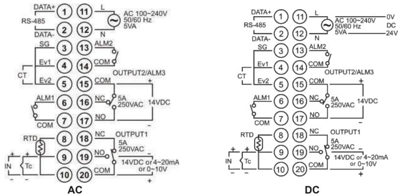
**Wiring for 4 to 20 mA Transmitter Inputs**
