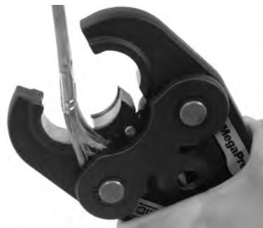
Figure 13 – Cleaning Segment Area of MegaPress Jaw
