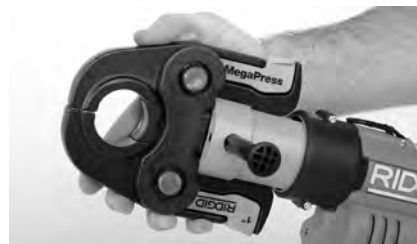
Figure 4 – Sliding The Attachment Out of the Tool
