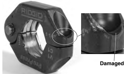
Figure 11 – Damaged Ring Pocket
