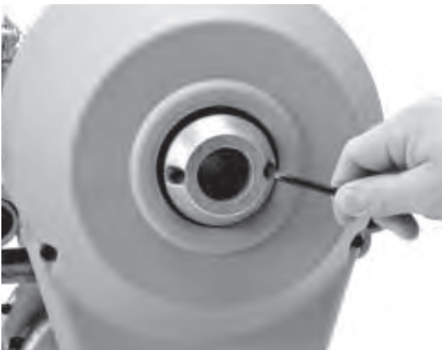
Figure 11 – Replacing Clutch Jaws
