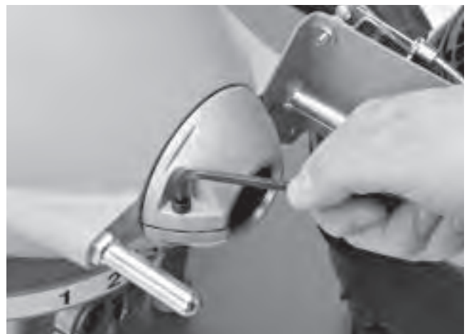
Figure 13 – Removing Clutch End Play
