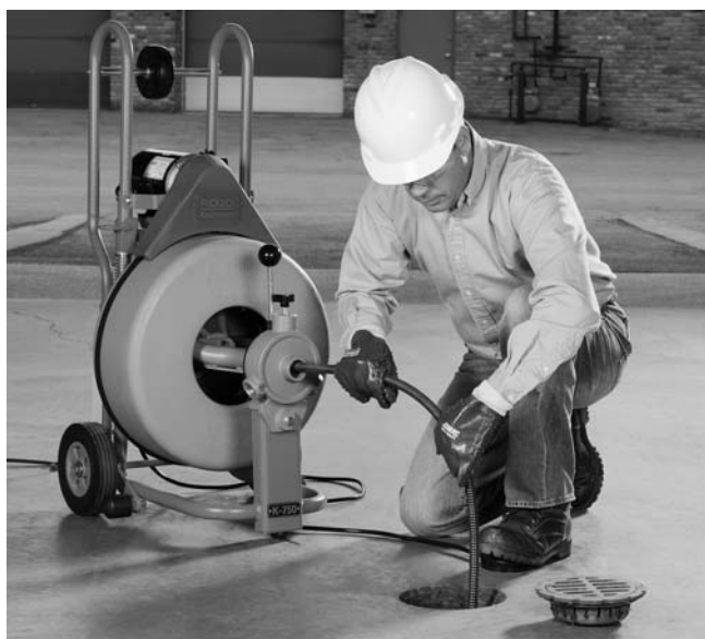
Figure 12 – In Operating Position, Manually Feeding Cable
