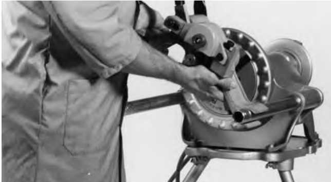
Figure 2 – Mounting on No. 300 Power Drive
