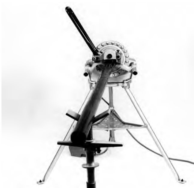
Figure 8A – Operating Machine in REVERSE (REV) Position
