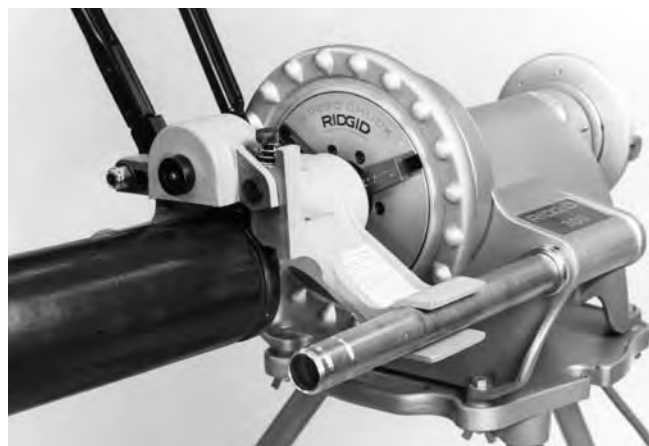
Figure 9 – Feed Handle in UP Position
