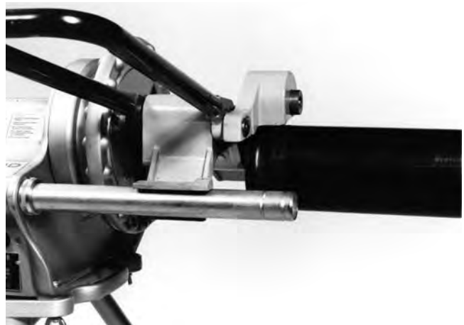
Figure 6 - Square Pipe & Pipe Support
