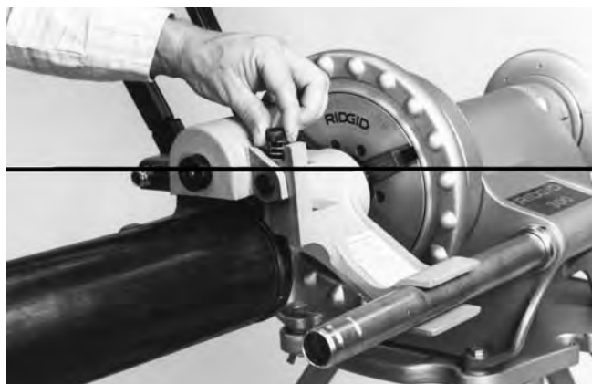
Figure 11 – Tighten Depth Adjustment Screw
