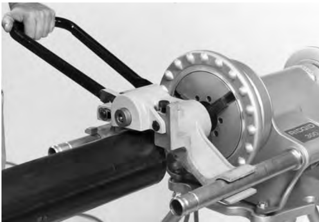
Figure 12 – Forming the Roll Groove
