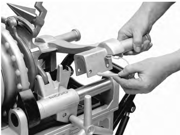
Figure 5 – Attaching Adapter Bracket to 300 Compact Threading Machine
