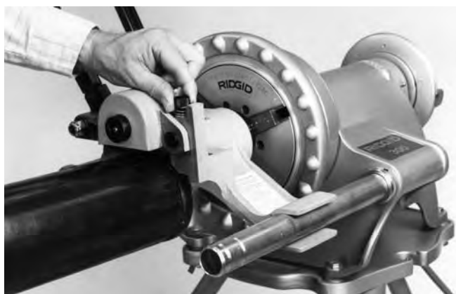
Figure 10 – Loosen Depth Adjustment Screw
