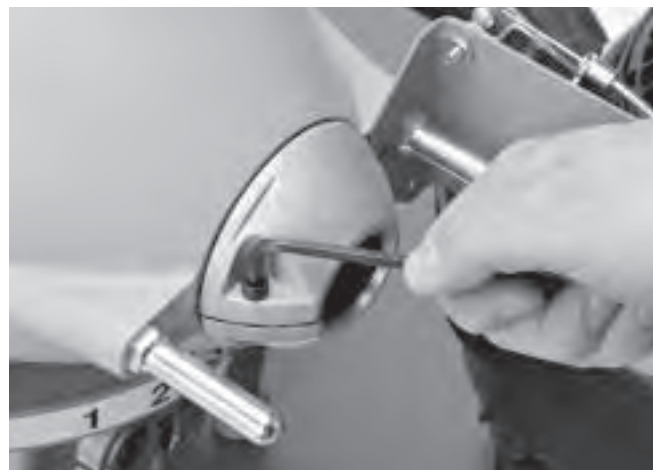
Figure 13 – Removing Clutch End Play
