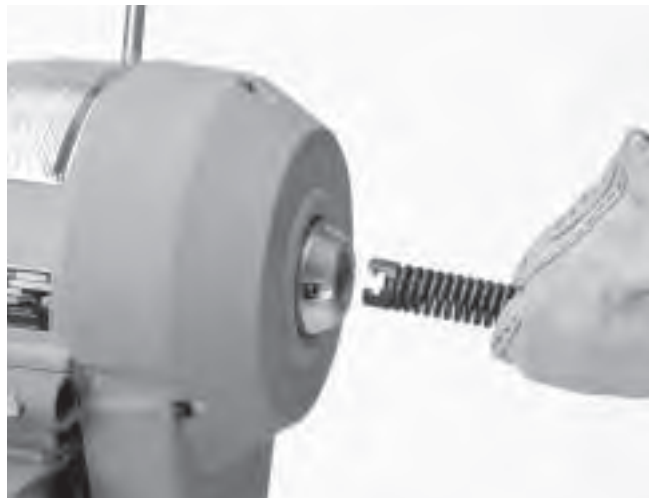
Figure 3 – Inserting Cable Into Front Of Machine
