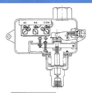
444-10 temperature switches with standard (13%" dia.) bellows will have differential characteristics at the high end of the range similar to those of a B-1 pressure switch (1°F = 1 PSI). 444-32 temperature differentials with standard (3/4" dia.) bellows compare with a B-6 pressure switch with some exceptions per MIL-S-16032. As a general rule, differentials at the low end of a temperature range are two and one half (21/2) times greater than at the high end of the range.
