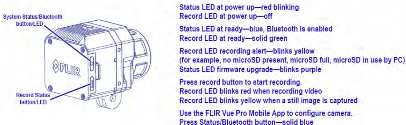
Figure 9. Camera Status and Record LED Description
