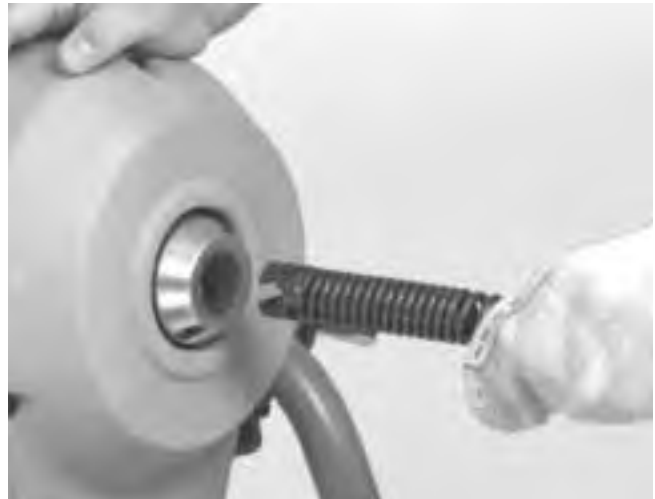
Figure 4 – Inserting Cable Into Front Of Machine
