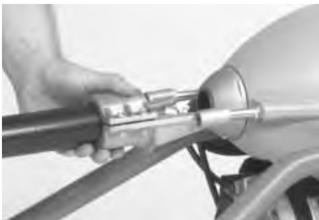
Figure 3 – Rear Guide Hose Attachment
