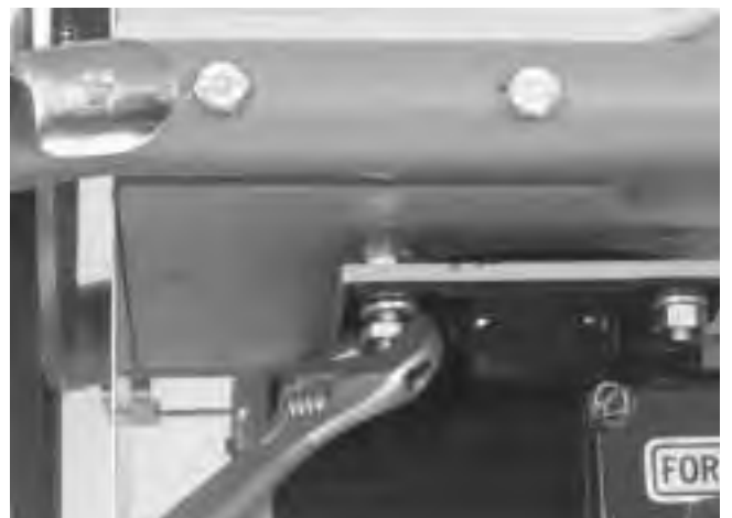
Figure 14 – Removing Clutch End Play
