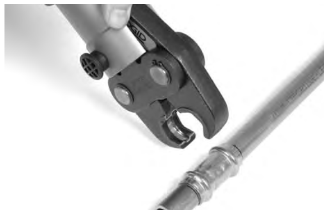
Figure 6 – Opening The Scissor-Style Jaw Set
