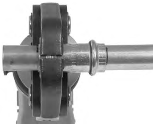
Figure 7 – RP 340 Tool Square To Tubing
