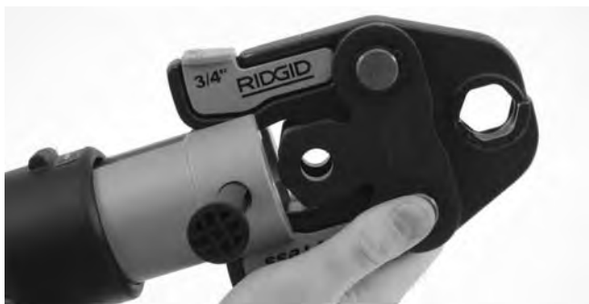
Figure 5 – Slide Attachment Into Tool
