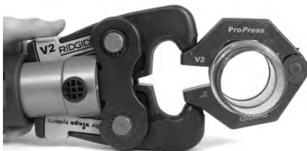
Figure 9 – Attaching Actuator to Press Ring
