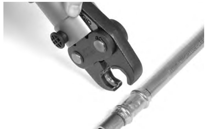
Figure 6 – Opening The Scissor-Style Jaw Set
