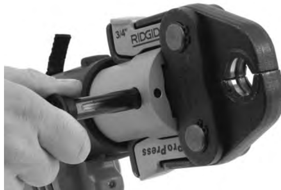
Figure 4 – Fully Open Attachment Mounting Pin
