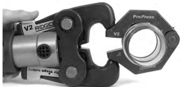
Figure 9 – Attaching Actuator to Press Ring
