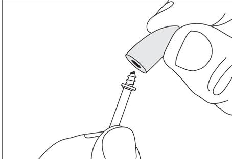
**Mandrel No. 401** is used with the felt polishing tip and wheels. Thread the tip on to the screw carefully. The felt tip must thread
