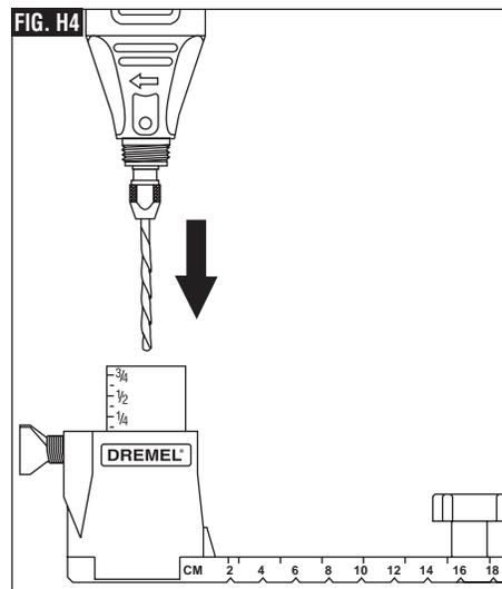
housing, thread the circle cutting guide onto the threaded portion of your Rotary Tool clockwise until tight. Do not hold the attachment by the metal rail during installation. Do not overtighten (Fig. H4).
