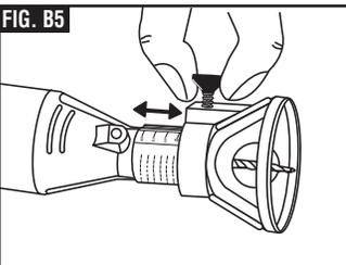
using the #560 bit you will be able to cut in a counter clockwise direction because the bit has a piloted tip and won't cut into the outlet box. The maximum cutting depth is 3/4" (19 mm). Thicker materials may require a slower, steadier cut. The recommended tool speed for the Drywall Cutting bit is generally 25,000-35,000 rpm. Caution should be used when making overhead cuts so debris is not getting drawn into the tool.
