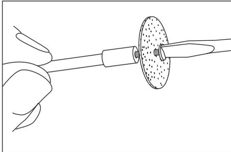
**Mandrel N° 402** has a small screw at its tip, and is used with emery cutting wheels and sanding discs. Higher speeds, usually
