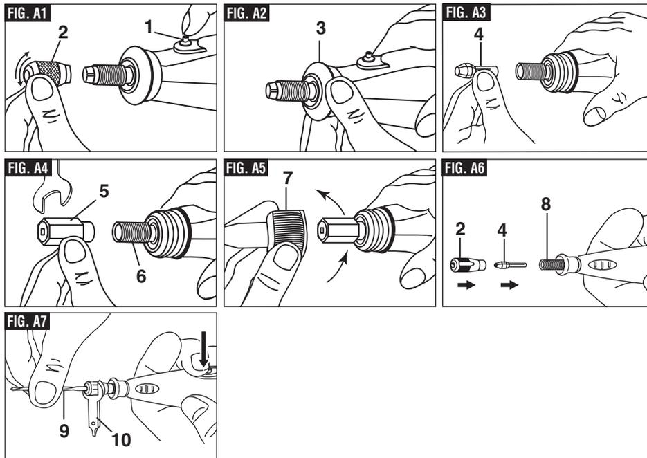
2. Unscrew the nose cap 3 from the tool (Fig. A2).
