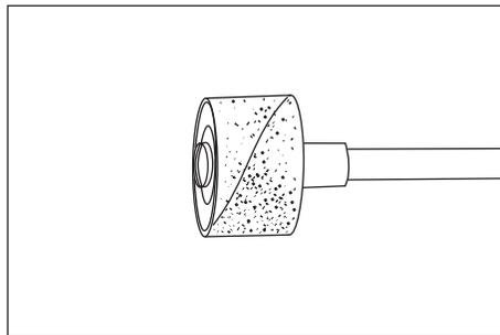
**⚠WARNING** Before each use, check to make certain that all components are assembled to accessory shank and that the drum is sufficiently expanded to secure the band during use. If sanding band is loose on the drum during operation it may “fly” off and strike you or bystanders.
