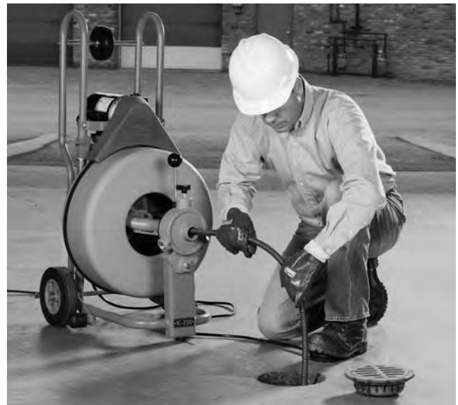
Figure 12 – In Operating Position, Manually Feeding Cable
