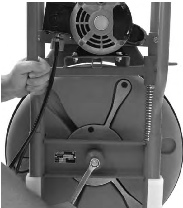
Figure 18 – Removing Drum Bolt
