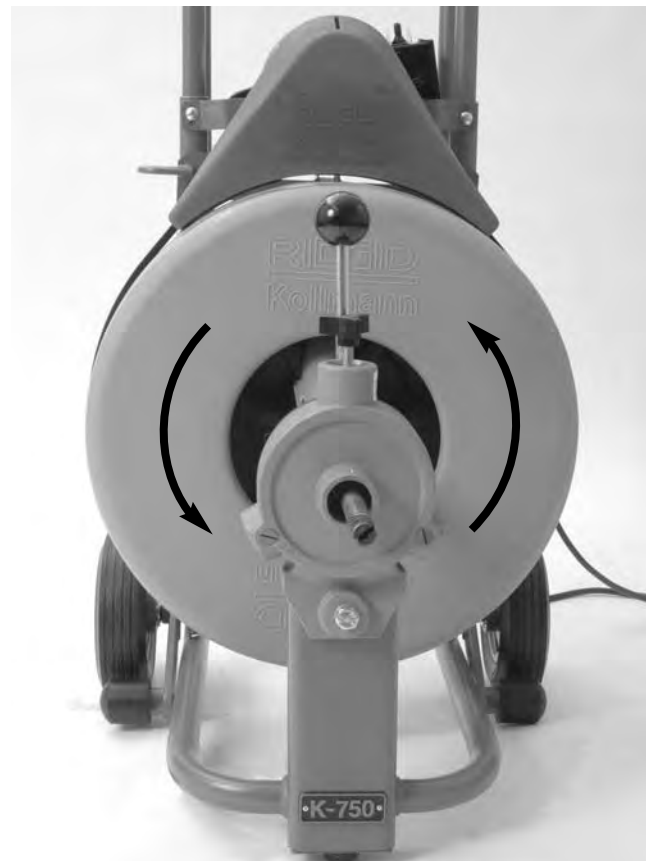
Figure 8 – Proper Drum Rotation (FOR Switch Position)
