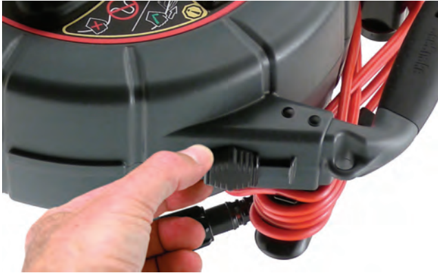
Figure 4 – Unlatching the nanoReel Case
