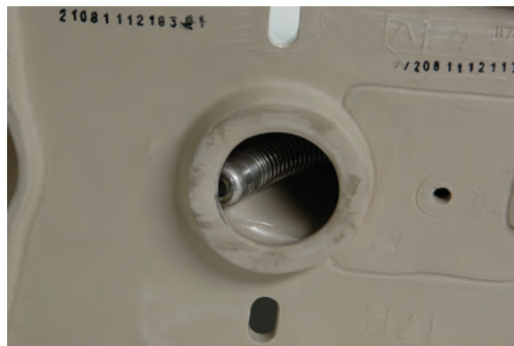
Figure 17 – Camera Head Blocked in Turn
