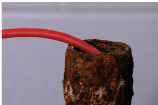
Figure 16 – Avoid Pulling at Sharp Angles
