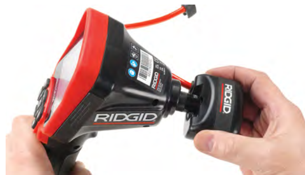
Figure 10 – Connecting the micro CA-300 Camera Monitor
