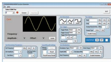
The signal generator can be programmed remotely via the USB (virtual COM) interface using SCPI commands. B&K Precision also offers application software (available for download at [www.bkprecision.com](http://www.bkprecision.com)) that provides virtual front panel emulation, allowing users to remotely control their instrument without the need for programming.
