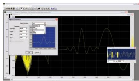
Use waveform editing software to easily generate, edit, and download custom arbitrary waveforms. Generate waveforms by importing a text file, or define via freehand, point draw, or waveform math. Waveforms can also be loaded from the generator for documentation purposes.
