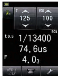
⑯ [Flash Duration Analysis Cord Mode Measuring screen]
