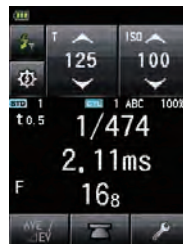
⑰ [Flash Duration Analysis Radio Triggering Mode Measuring screen]
