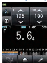
⑪ [Radio Triggering Flash Mode Measuring screen]
