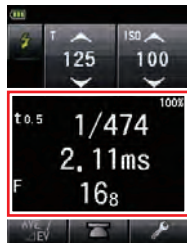
[Flash Duration Analysis Cordless Mode Measuring screen]
