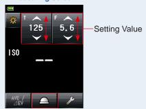
**6.** Press the Measuring Button **6** to measure the light on the side of the meter.
