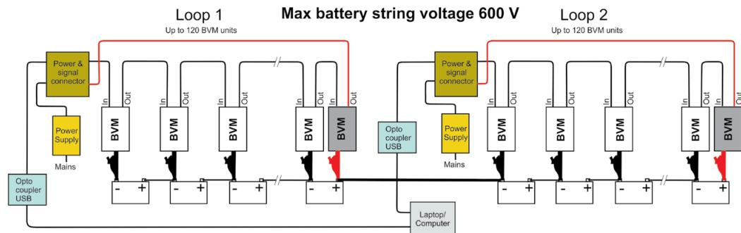
When the battery bank voltage exceeds 500V, Torkel cannot be used. Instead the voltage measured from the cell/block can be monitored from a PC using PowerDB or Torkel Win report sw. This require use of 2 pcs. opto couplers ( Art no HC-50040 ) and 2 pcs. ungrounded power supplies ( Art no HC-04155 ) for each loop. Each loop not to exceed 300V.
