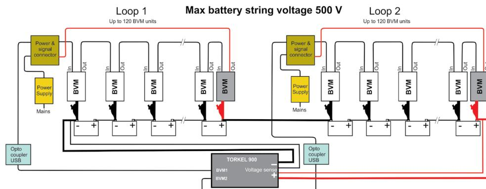
The connection shown above must be used when the battery bank voltage is between 300 V and 500 V. It includes two opto couplers and two ungrounded power supplies.
