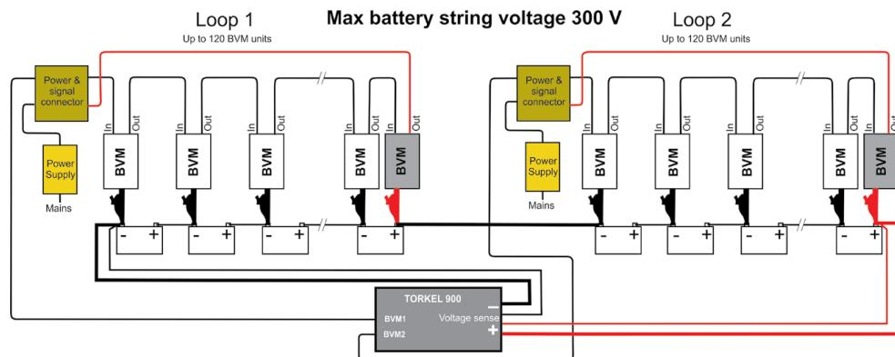
When the battery bank exceeds 120 cells, connection with 2 BVM loops shall be used.
