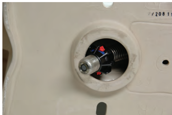
Figure 18 – Camera Head with Ball Guide in Turn
