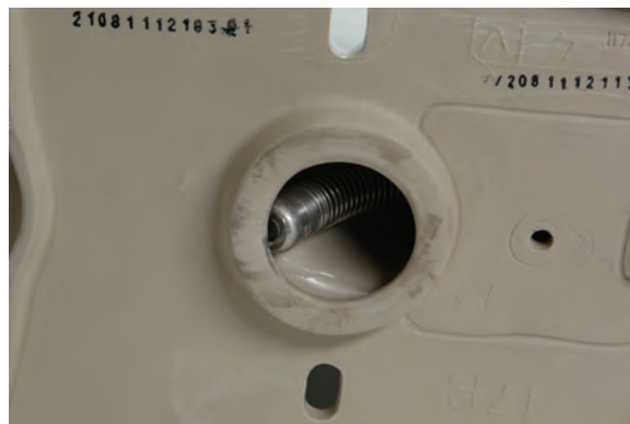
Figure 17 – Camera Head Blocked in Turn
