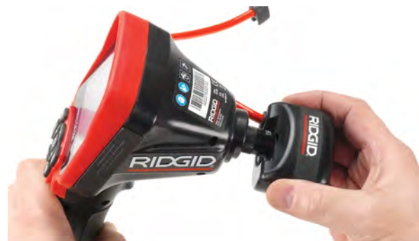
Figure 10 – Connecting the micro CA-300 Camera Monitor
