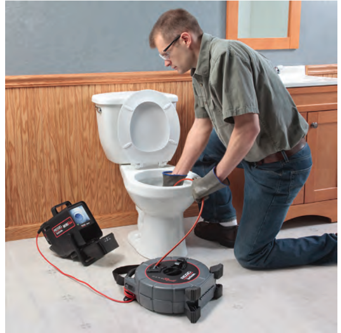
Figure 14 – Performing an Inspection
