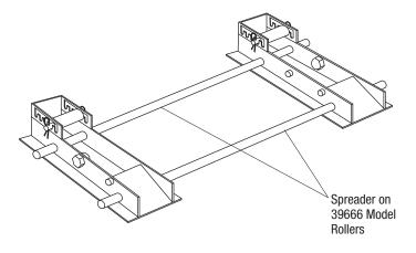
2. Secure the reel roller to the floor using 1/2" or 3/8" bolts.
