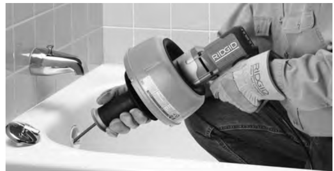
Figure 9 – Push Cable Down Drain Line
