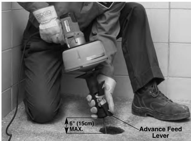
Figure 10 – Feeding Cable With AUTOFEED
