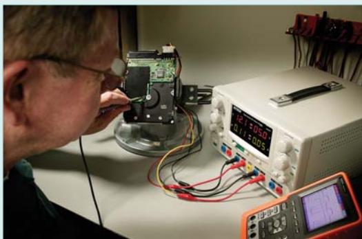
Single power supply with multiple DC outputs
