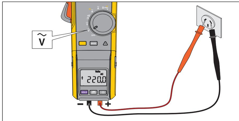
Figure 6. Measurement with Test Leads (AC Voltage Shown)
