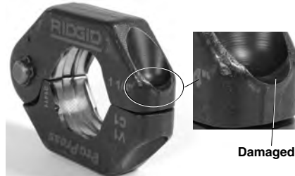
Figure 11 – Damaged Ring Pocket
