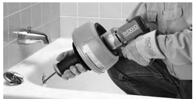
Figure 9 – Push Cable Down Drain Line
