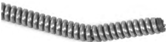
Figure 15 – Bend At Cable End
