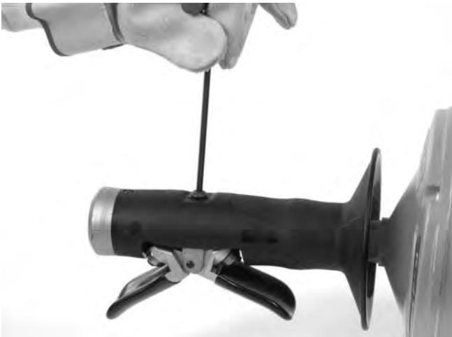
Figure 12A – Removing AUTOFEED Screw
