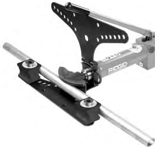
Figure 10 – Loading the Pipe
