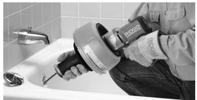
Figure 9 – Push Cable Down Drain Line
