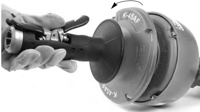
Figure 14 – Twist Drum Apart
