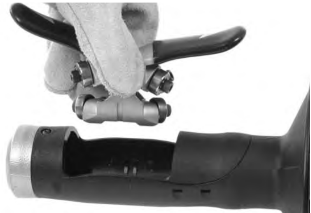
Figure 12B – Removing AUTOFEED Mechanism From Housing
