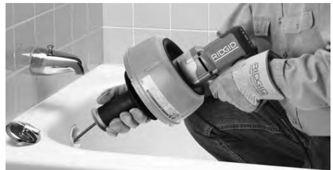
Figure 9 – Push Cable Down Drain Line
