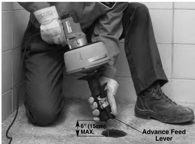
Figure 10 – Feeding Cable With AUTOFEED
