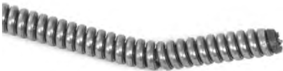
Figure 15 – Bend At Cable End
