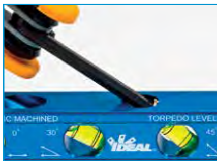
4. Reinstall O-ring and set screw
