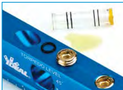
2. Remove O-ring and damaged vial
