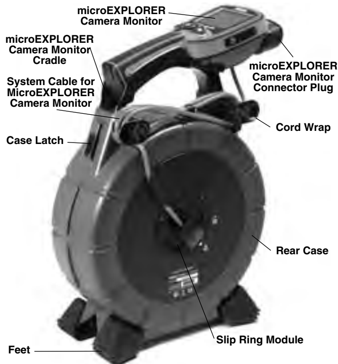
Figure 2 – Rear View (microEXPLORER Camera Monitor Configuration)
