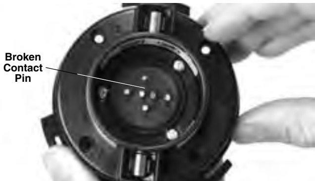
Figure 7 – Broken Contact Pin
