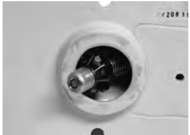
Figure 21 – Camera Head with Ball Guide in Turn
