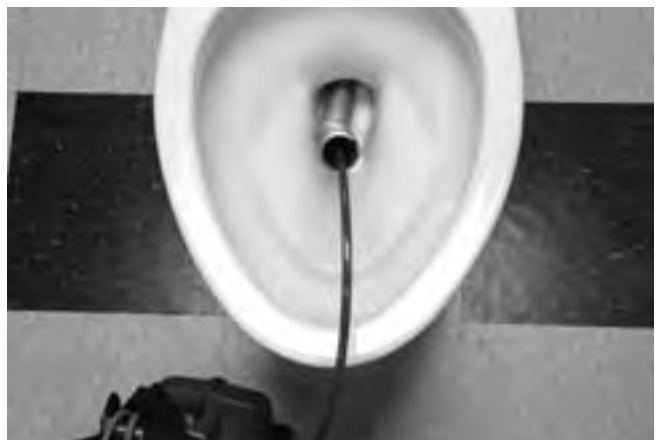
Figure 25 – Using The Flexible Guide Tube
