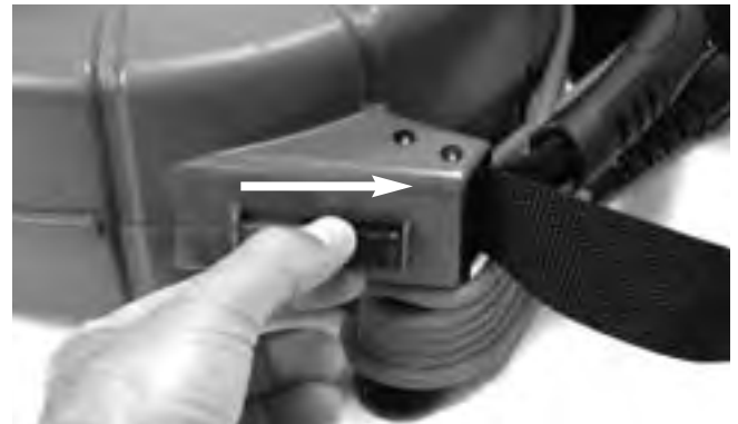
Figure 4 – Unlatching the microDrain Reel Case
