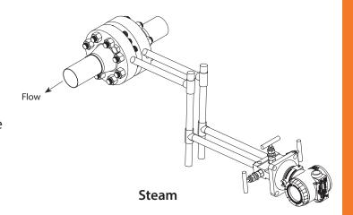
**Note:** For steam or other elevated temperature services, it is important that temperatures at the process connection do not exceed the transmitters process temperature limits.
