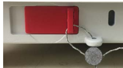
Locked with Wire Seal
