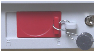
Locked with Wire Seal
