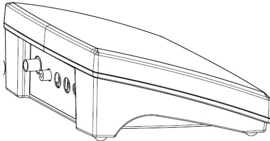
For ST310 electrode connect to the BNC and Cinch socket. For 2-in-1 pH electrode (e.g. ST210) you only need to connect to the BNC. Temp. socket is for a separate temperature electrode.
