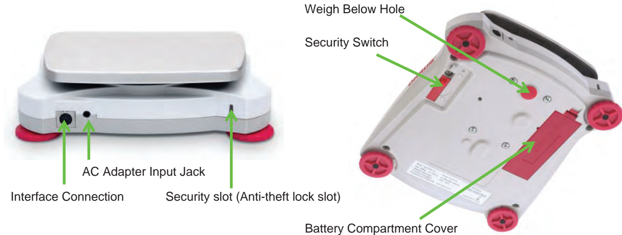
Figure 2-3. Rear and bottom view of balance
