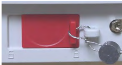
Locked with Wire Seal
