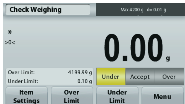
The Check Weighing Home screen
