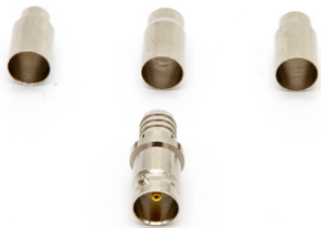
350-00-75TP Universal BNC Female 2 Pc Crimp-On, 75 Ohm
