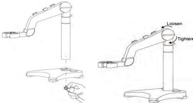
After adjusting the tension knob to some extent, you can move up and down. When the electrode is installed on the arm, the storage bottle of pH electrode fits into the base hole.
