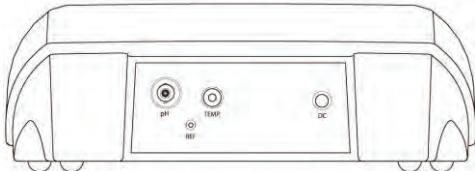
For ST210, you only need to connect the pH electrode with the pH socket (BNC);
