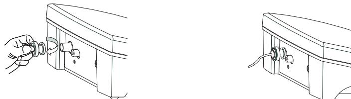
For temperature electrode STTEMP30, connect with Temp. Socket (Cinch).
