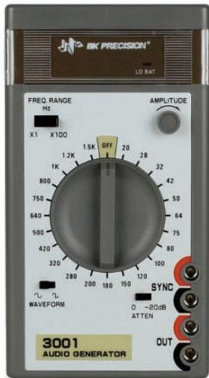
The model 3001 generates low-distortion sine waves at 46 discrete frequencies. Output impedance is  $600\ \Omega$  at the dual banana jacks and the output voltage is continuously adjustable up to 1.2 V (RMS) into an open circuit. Output flatness is  $\pm 0.5$  dB. A 5 Vpp square wave is provided at separate banana jacks for synchronization. Frequency accuracy is 3% from 20 Hz to 100 kHz. The unit is powered by a 9 V battery.
