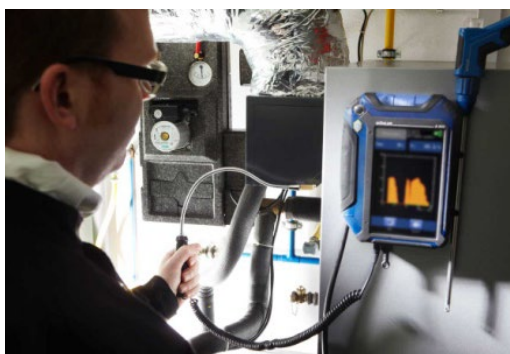
Fig. 51: Spillage test: Searching for condensate
