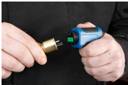
Fig. 24: Connecting the probe
