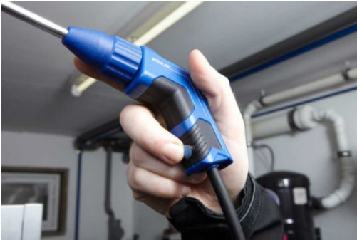
Fig. 5: Pressing the ON/Off-Key during the measurement
