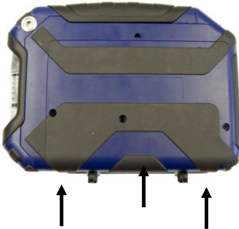
Fig. 72: Bottom of the unit - Press to open the cover.
