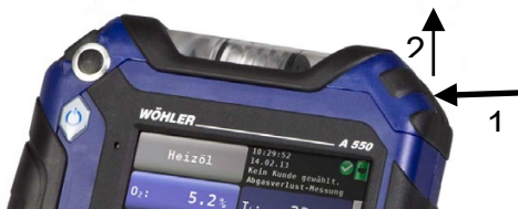
Fig. 67: Open the condensate trap compartment
