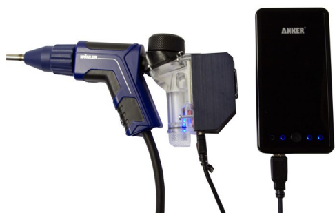
Fig. 60: Probe grip with Peltier Cooler and USB power bank
