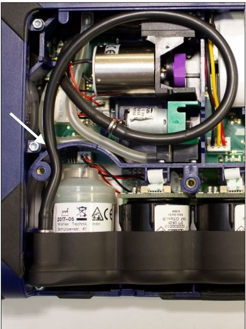
Fig. 77: Connecting tube, correctly positioned
