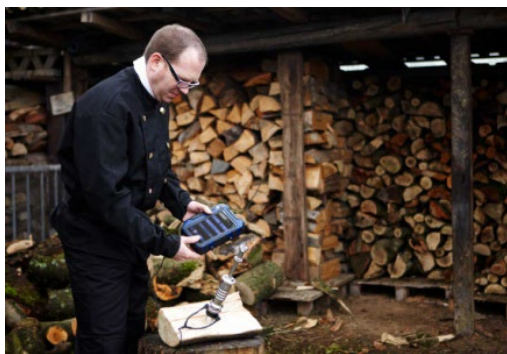
Fig. 46: Wood moisture measurement with Probe Wohler HBF 420.
