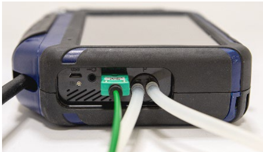
Fig. 38: Analyzer with pressure hoses and temperature plug
