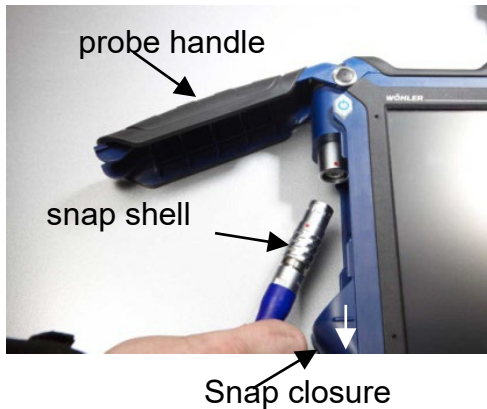
Fig. 27: Wohler A 550 INDUSTRIAL with open probe compartment
