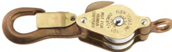
This block features an eye to splice line to block and rope tie-off. Made of light galvanized steel and aluminum alloy. The sheaves have bronze bushings for long life.
