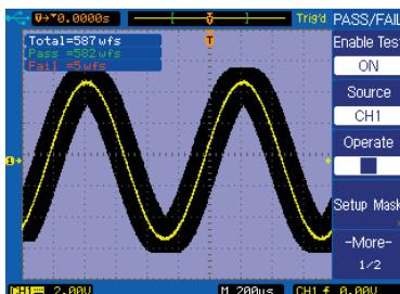
Generate user-defined pass/fail limits to quickly identify go/no go test results.
