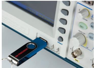
Save and load arbitrary waveform data in CSV format from a USB flash drive.
