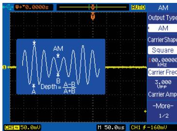
Display a graphical illustration explaining the parameters of the built-in arbitrary waveforms and modulation schemes. This is a convenient tool for students and new users.
