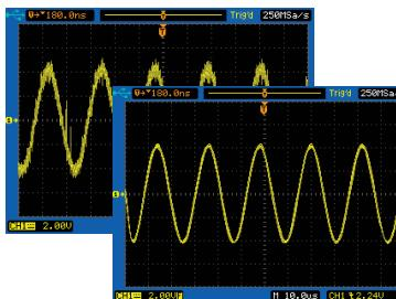
Filter out unwanted signal components such as various types of noise with built-in digital filters. Choose from Low-Pass, High-Pass, Band-Pass, and Band-Stop filters.
