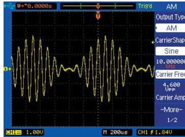
The built-in arbitrary waveform generator is capable of many different types of modulation for various applications. Modulate your waveforms with AM, FM, FSK, PSK, and PWM modulation schemes and use any of the 30 built-in waveforms as the modulating waveform.
