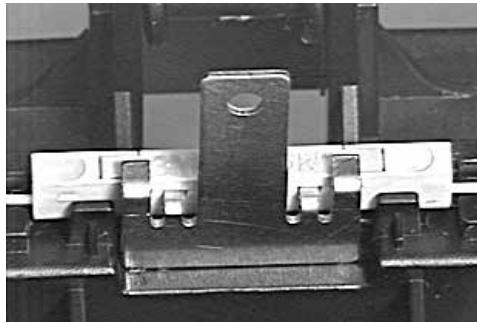
5.4 Hold the cap lifter in place with one hand and push down on the ends of the splice with the other hand. This action should reseat the splice into the holding cradle and lift the cap at the same time.
