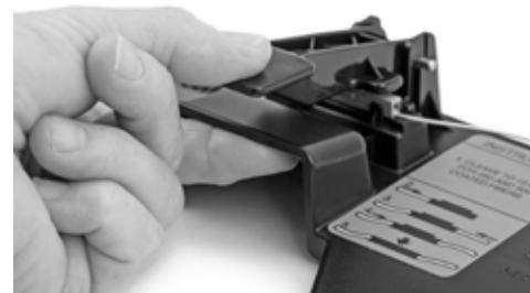
4.10 Remove the 3M Fibrlok Splice from the assembly tool by first removing the fibers from the foam retention pads and then lifting the splice from the splice holding cradle.
