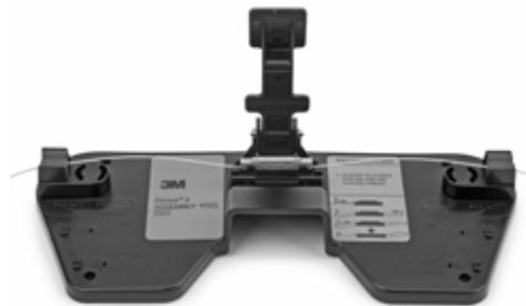
4.9 Pivot the handle of the 3M™ Fibrlok™ Assembly Tool 2501 down until it contacts the cap of the Fibrlok splice. **Squeeze the handle of the assembly tool as shown in order to close cap and actuate the splice. When possible, secure the tool to a work surface for added support.** A snap sound will be heard when the splice is actuated.
