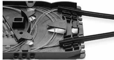
6.4 Place the splice assembly tool close to or on top of the splice tray. Match the orientation of the tool to that of the splice holder or tray whenever possible.
