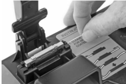
**Note:** Push fiber straight into fiber alignment guide, NOT AT AN ANGLE.
