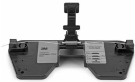
4.8 Push the first fiber back against the second fiber until there are equal bows in both fibers.
