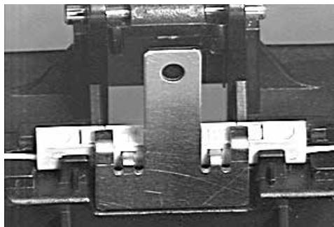
5.3 Slide the bottom of the cap lifter inward until it is in a vertical position, lifting the splice slightly out of the cradle.
