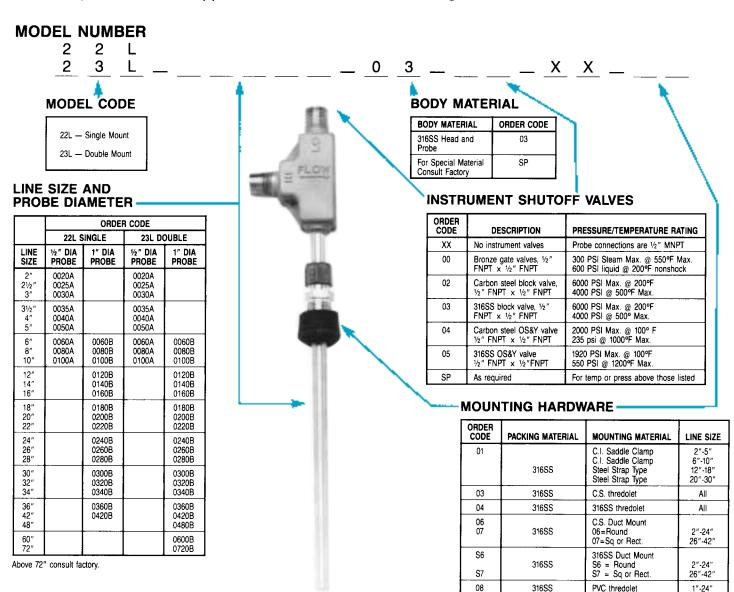
SERIES 22L—ACCUTUBE—SINGLE MOUNT. The Accutube Series 22L Probe is constructed of 316LSS cast head and 316LSS probe. The Series 22L probe has single-mounted support and installs through a single packing gland and thredolet. The Series 22L Accutube is factory-fitted with ½" NPT connections and is shipped with mounting hardware complete. Series 22L Accutubes are available for line sizes 2" through 42".
